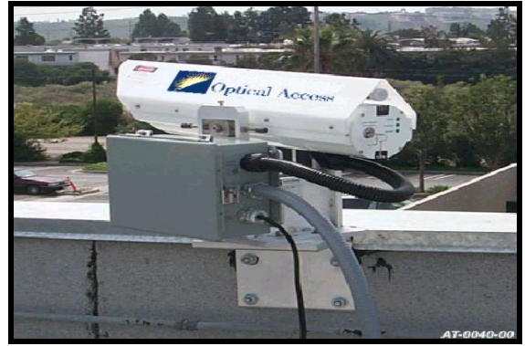
Figure 2.11: Angle Bracket Mounting (using JMP and M001)
